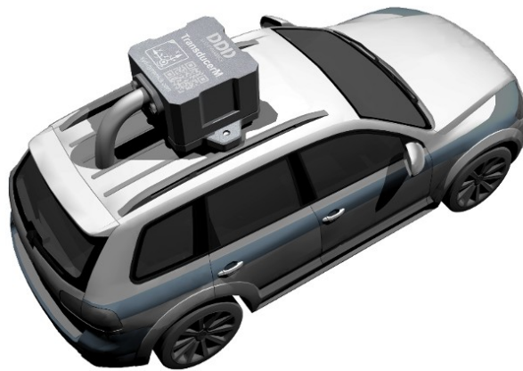
Figure 10: Example Install of a TransducerM on a Model Car (Not drawn to scale). The X-Axis points to the forward direction.
